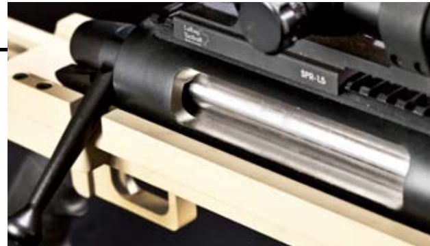
The Halo Maximus uses a BAT Machine receiver and locks via two massive lugs at the front, spaced opposite from each other. The bolt handle can be considered as safety lug, and the Maximus' bolt operation was butter-smooth right from the box.
