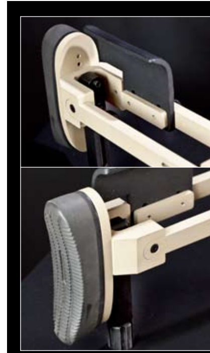
The stock is machined from 6061-T6 billet aircraft aluminum, hard anodized to military specifications and has a hook on the toe of the butt that allows the shooter to pull the rifle really tight into the shoulder – a necessity when shooting a large caliber rifle.
